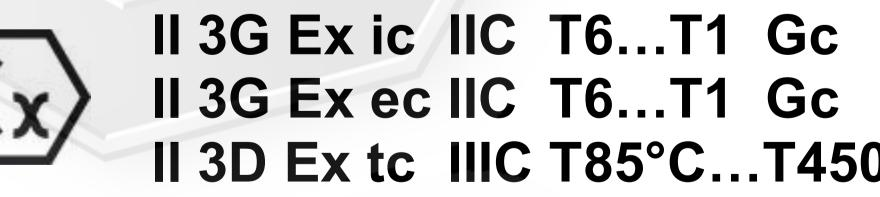
II -/3G Ex ic IIC T6...T1 -/Gc II -/3G Ex ec IIC T6...T1 -/Gc II 3D Ex tc IIIC T85°C...T450°C Dc II -/3D Ex tc IIIC T85°C...T450°C -/Dc
