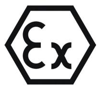
2G Ex eb IIC T6...T3 Gb 2D Ex tb IIIC T85°C...T200°C Db
